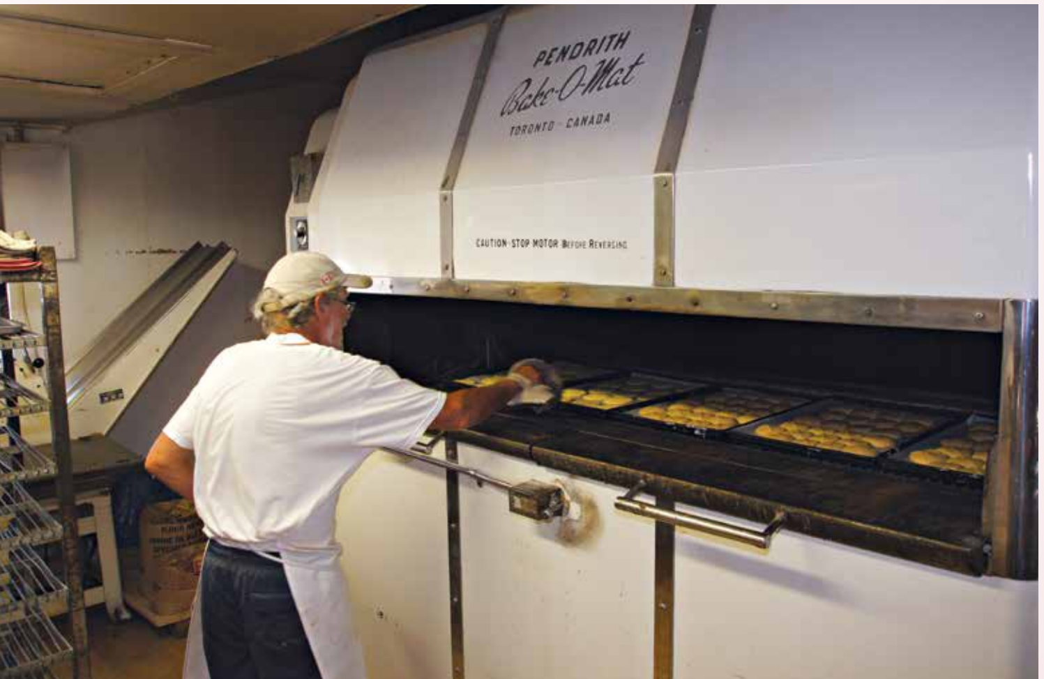
▲ The baking is done. Paul Holman putting his hand into the mouth of the oil-fired Pendrith Bake-O-Mat.
